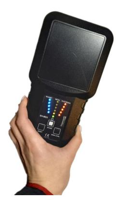
The **Switched-On electronic devices detector** channel can be used to find the different types of switched-on electronic devices, namely digital timers and remote-control units, photo and audio/video recording devices, laptops, touchpads, cell phones of all standards (also in a sleeping mode) and etc. The principle of operation is based on the registration of the magnetic field pulses generated by the current pulses of switched-on electronic devices.
